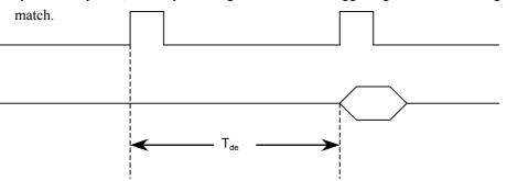
$T_{de}$ : The external trigger signal is the delay time for burst signal output, the time from the trigger signal to the rising edge of the first slot of the frame.
