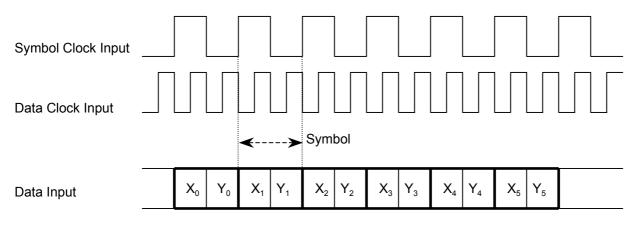
A Symbol consisting of  $X_n$  and  $Y_n$  where  $X_n$  indicates preceding data. When inputting one or two of the signals above, align the timing to the output signal of the signal that is not input.
