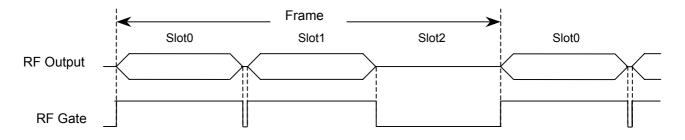
Slot details are shown in the figure below. The slot format in the figure is a sample for description and differs from that of the actual system.
